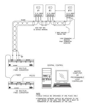
Figure 2: RS232 to FIBER and FIBER to RS485
